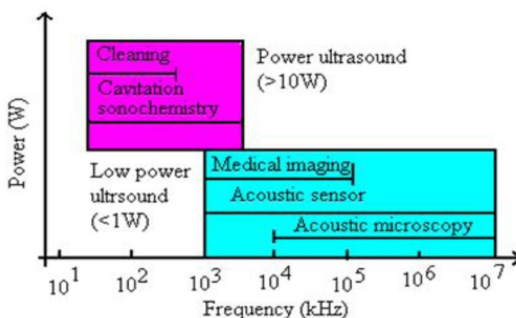
**Figure 3:** Power versus frequency
