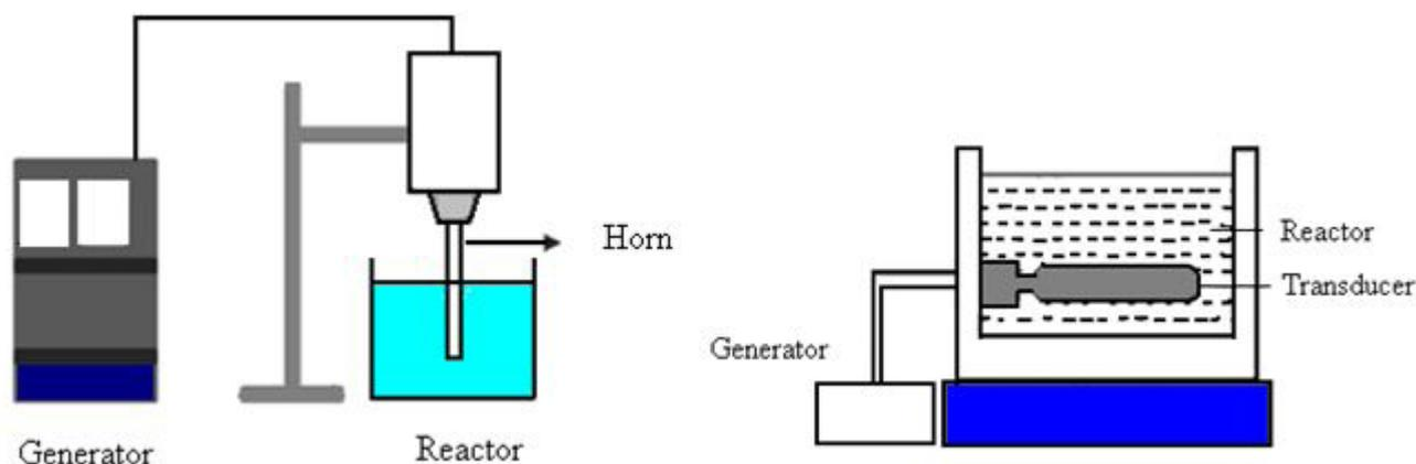
**Figure 2:** (a) Probe type sonicator (b) longitudinal horns
