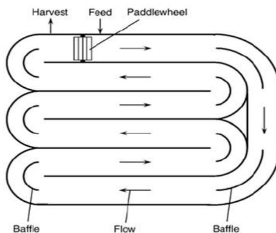
**Figure 6:** Aerial view of raceway pond
