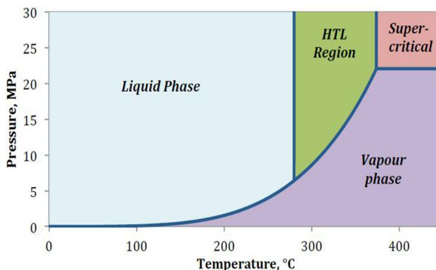
**Figure 9:** Hydrothermal Liquefaction
