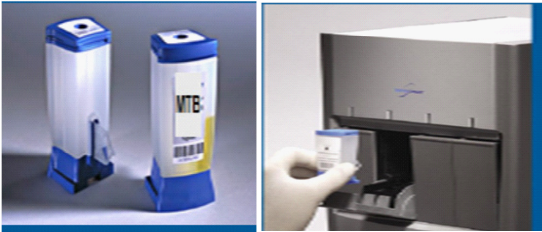
Figure 7: GeneXpert- MTB RIF Test showing cartridge and instruments
