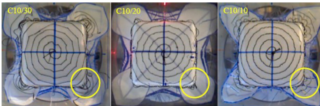
Figure 11: Top view of the deformed preforms with different tufting density [69].
